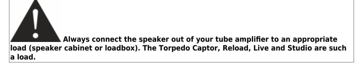
Please note that you must always power up the Torpedo Reload, Live and Studio before your amplifier, because the loadbox embedded in these products is only active when they are powered up. The Torpedo Captor does not need to be powered up to act as a loadbox.
