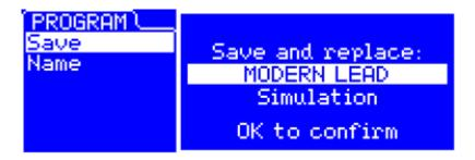
• Save: Press "OK" to display the saving screen for the current preset. Choose the saving destination from the 100 at your disposal, using the "NAVI" knob. Press "OK" again to save the preset.
