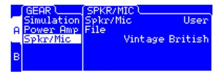
• **User:** Determine which impulse response (IR) file to use for the simulation.
