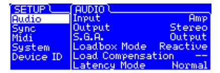
• Input Select: Select the input you want to activate for processing. The various routing options
