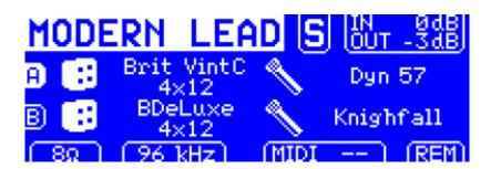
The mode of the selected preset (**Simulation** or **Arcade**) is displayed via either an **S** or **A** towards the top right corner.
