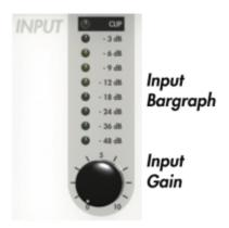
This potentiometer controls the SPEAKER input gain of the unit. The Torpedo Studio being a digital product, it is absolutely critical that you avoid any saturation of the input signal, or you may considerably reduce the sound quality. To get the best sound, try to have the same volume (or close) on all different sounds coming to the Torpedo Studio.
