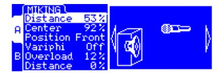
• Determine the distance between the simulated cabinet and microphone. Placing a microphone close to the cabinet will result in a precise sound with a large amount of proximity effect (dependent on the chosen model of microphone).
