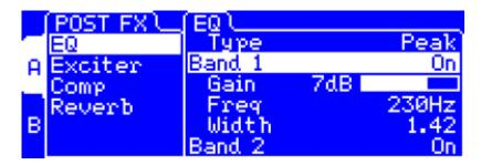
The 4 middle bands are peak filters with the following parameters:
