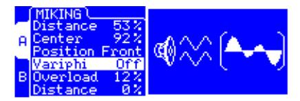
The Variphi function allows you to play with the phase of the signal. When recording with two
