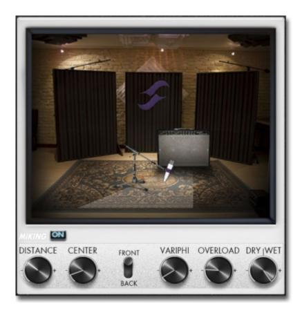
In the "MIKING" menu, you take the place of the sound engineer. This is where you will find the "sweet spot", the perfect microphone position. You will also be able to control speaker saturation and balance between simulated and non-simulated tones. The first two parameters determine the microphone's position. You can move the microphone around inside a trapezoidal plane that the Torpedo Remote software lets you visualize.
