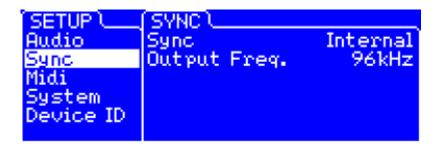
• **Sync:** The Torpedo Studio can be synchronized with an external clock ("Wordclock") or with input digital signals ("S/PDIF" or "AES/EBU"). If you select an external clock sync, the detected frequency ("Output Freq.") will be in the Sync menu when the Torpedo Studio is actually locked
