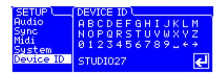
• **Device ID:** This menu lets you give an identifying name to your machine. If you wish to use the Torpedo Remote software to control several different machines simultaneously USB-connected to the same computer, you will have to give each machine a different Device ID. Move through the alphabet using the "NAVI" knob and select the letters with "OK".
