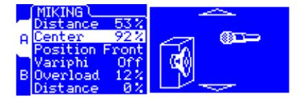
• Determine the distance between the axis of the loudspeaker and the microphone (placed at a right angle). The in-axis position (0%) allows for a maximum amount of trebles, which are highly directives.
