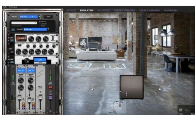
The Simulation mode gives you access to all parameters and the two microphones, which can be placed at the front or the back of the cabinet.
