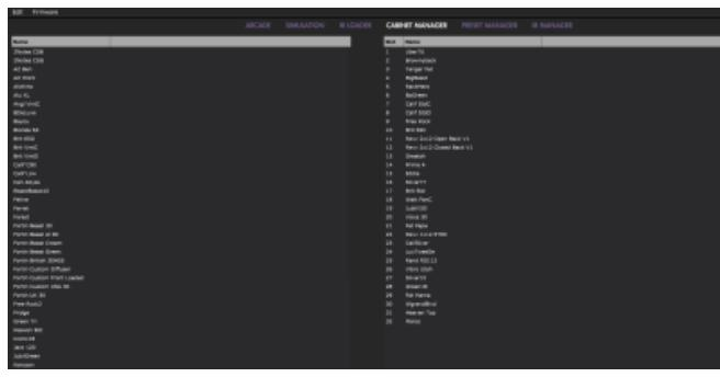
In the Cabinet Manager window, you can visualize on the left side the cabinets that are available in your license and on the right side what cabinets are loaded in the pedal. You can drag and drop your cabinets from the left side panel (the computer side) to your Torpedo (the right side panel). If ever the 32 memory slots are full in the Torpedo, you need to free space by dragging and dropping any cabinets to the bin.
