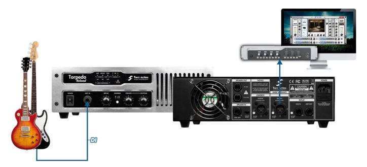
In any setup that involves a microphone preamplifier, it is important to set the correct gain on the preamplifier so the level of the recorded track is high enough. It is commonly recommended to set the gain on the preamplifier so the instrument's signal will hit -16dB FS to -18dB FS (i.e., dB Full Scale, the value indicated on your sound card and sequencer input meter).
