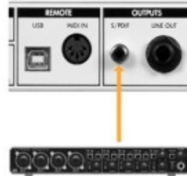
Plug your 8 ohms out on your amplifier to the SPEAKER input of the Torpedo Live. Connect the S/PDIF OUT of the Torpedo Live to the S/PDIF IN of your audio interface. The sampling frequency can be set to 48KHz or 96KHz.
