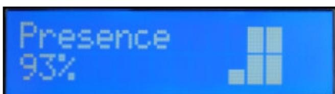
This setting affects the tube stage frequency (loudness), by giving more low end to the signal. The depth at 0 does not affect the incoming signal, while at 1000 the low end frequencies are boosted.
