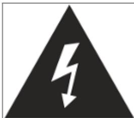
The triangle with a lightning bolt means that some parts of the product, even when the power is turned off or unplugged, can retain voltage high enough to cause serious electric shock. Any operation that requires opening the device should be left to a qualified technician.
