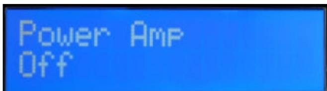
In Guitar mode we selected an EL34 Pentode PP power amp and a 6L6 Pentode PP power amp for Bass. Presence and Depth are fixed at 100%. The Power amp parameter determine the amp master volume, from Cold to Hot. it can also be turned OFF.
