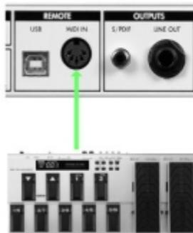
The Torpedo Live handles both Program Change et Control Change commands. See section 6 of this manual for the complete MIDI guide of the Torpedo Live.
