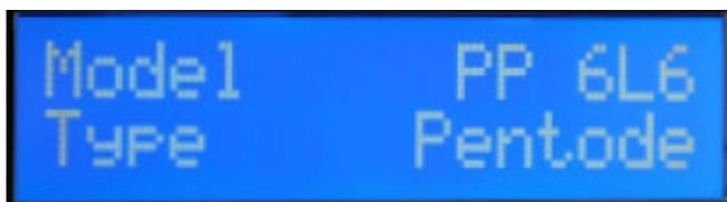
MODEL is the amplifier topology (Push Pull or Single Ended) and the tubes type (6L6, EL34, EL84 or KT88). TYPE selects how the tube is used, either in triode or in pentode mode. Pentode mode has more headroom and volume than triode.
