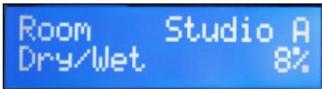
The room type determines the type of reverb you will apply to your guitar or bass tone. You have access to 8 different rooms: Studio A & B, Hall A & B, Cathedral, Crypt, Basement and Loft. The Dry/wet setting determines the amount of reverb to be applied to your tone.
