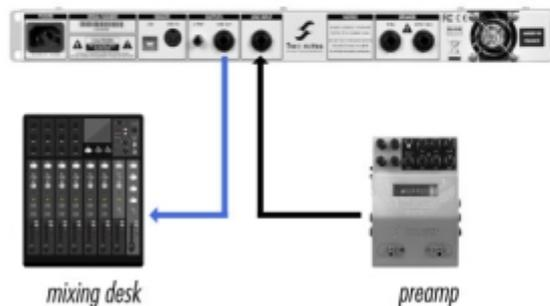
The Torpedo Live can be used with a preamp instead of an amp. To do so, connect the preamp to the Line Input of the Torpedo Live. The Line Input has priority on the Speaker input. Meaning, if a cable is connected to the Line Input, the Speaker input is disconnected.
