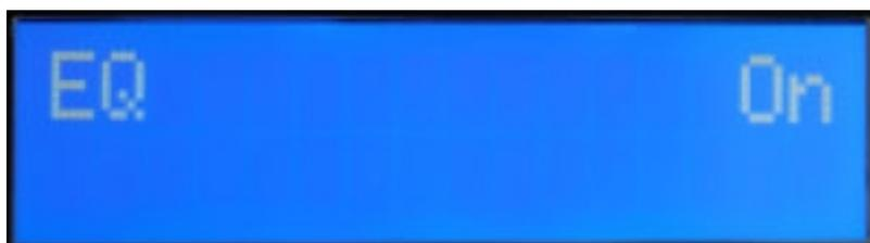
The equalizer (EQ) section is a simple yet powerful 5-band EQ. It has 3 mode of operations : guitar, bass and custom. Guitar and bass are centered around fix frequencies for each band, whereas custom mode is a semi parametric eq with an adjustable low cut filter.
