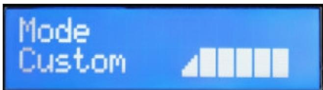
**Custom mode** : Instead of having fixed frequencies to work with, the Custom mode gives you access to a 6 band semi parametric EQ (12 dB per octave slope). The bands are as follow:
