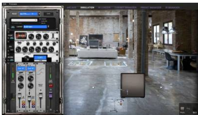
The Simulation mode gives you access to all parameters and the two microphones, which can be placed at the front or the back of the cabinet.
