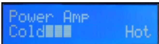
The Power amp parameter determine the amp master volume, from Cold (low power) to Hot (high power). it can also be turned OFF.
