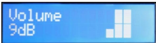
Set up the output volume of your virtual power amplifier. The volume at 0 is the same as switching off the Power Amp.
