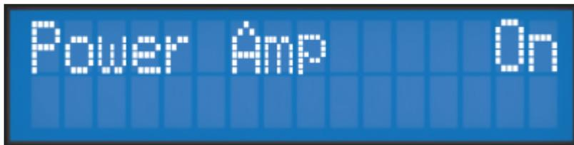
A module is activated when it's On, you can change the module state with the VALUE encoder. Once the module is On, you gain access to the module parameters.
