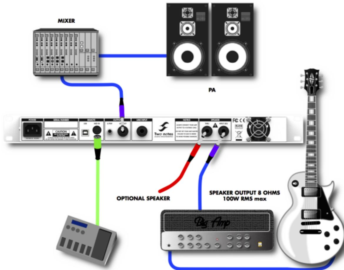
With a MIDI foot controller, you gain access to the presets navigation and even parameter changing in real time. The Torpedo Live handles both Program Change et Control Change commands.
