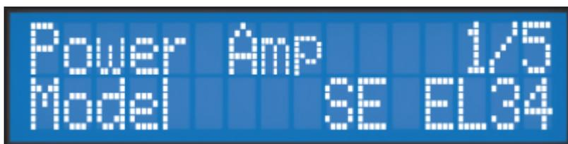
On a parameter page, you will see on the first line the module name, the parameter index and the number of parameters of the module. On the second line you will find the parameter name and its value. Change the value using the VALUE encoder.
