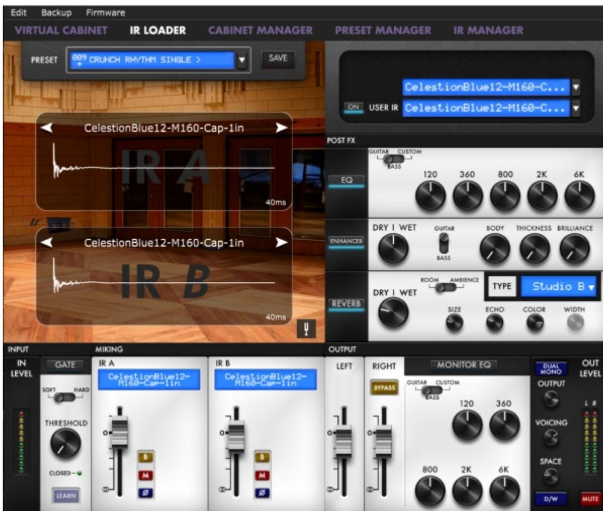
The Torpedo Captor X can load up to 512 IRs. All imports of IRs are done by Torpedo Remote through the IR manager (via computer). Upon upload into the Captor X, the IRs length can be set to 20, 40, 100 or 200 ms long. If the IR is longer it will be shortened by Torpedo remote to the selected length. If it is shorter it will be extended (filled with zeros) to the selected length. The internal memory has the following allowances regarding the length of the IR:
