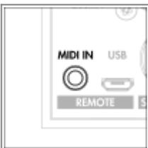
Torpedo Captor X can be controlled by MIDI, with any regular MIDI controller. To control the Torpedo Captor X via MIDI use the supplied MIDI to mini jack converter cable. You will be able to control any parameters of the Torpedo Captor X through Control Change, or change presets through Program change. You can see the MIDI mapping in the section of the owner's manual.
