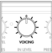
On the front panel of the Torpedo Captor X, the VOICING control allows you to adjust the global sound of the unit coming out of the XLR outputs. It is a simple one band equaliser that is centered at 900 Hz with a -12 to +12 dB range.
