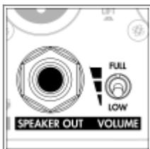
To use the attenuator, you need to connect a cabinet to the SPEAKER OUT of the Torpedo Captor X. You will activate the attenuator with the Volume Level switch.
