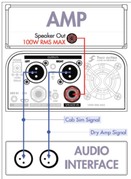
Connect your amp's output to the SPEAKER INPUT of the Captor X, indicated by a red bolt - ONLY use a speaker cable for this connection. In Torpedo Remote, select the DUAL/MONO routing and bypass the Torpedo Processing on the RIGHT output. The left XLR output will send the full Torpedo signal, while the right XLR output will send the dry signal of the amp to the interface, adding the cabinet simulation with Torpedo Wall of Sound in your DAW.
