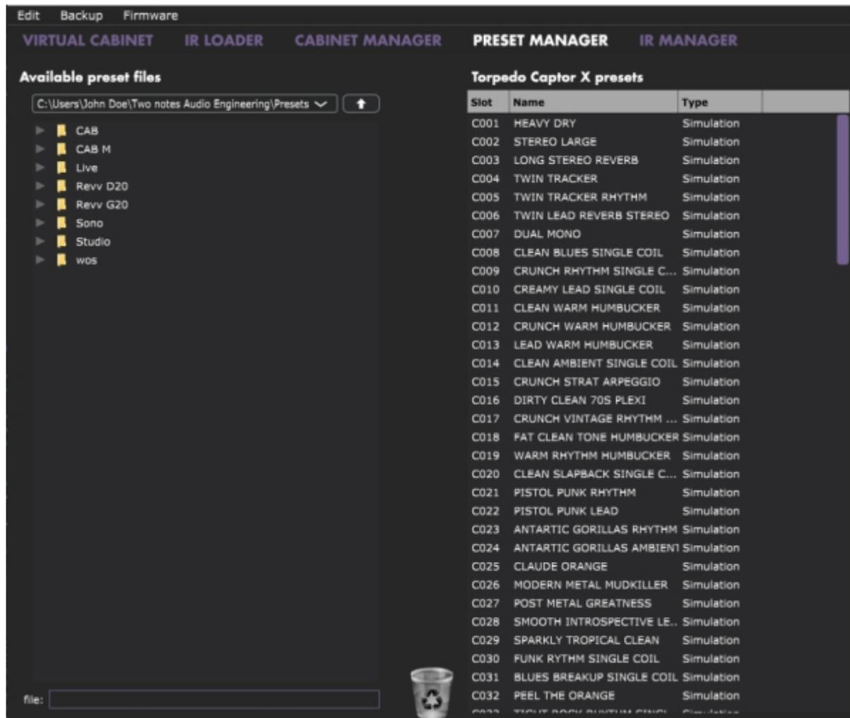
Move the presets up and down to change their order in Torpedo Captor X. The first 6 slots are accessible by the PRESET knob at the front of the unit. Remove presets by dragging and dropping them in the bin below. Drag and drop presets from the left panel (your computer) to the right panel (internal memory of the Captor X).
