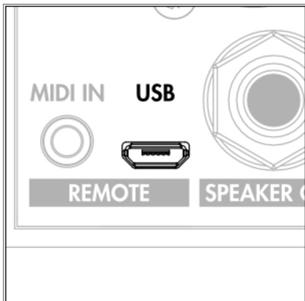
Use the supplied USB cable to connect the Torpedo Captor X to your computer. Connect the micro USB end to the Torpedo Captor X and the other end to your computer.
