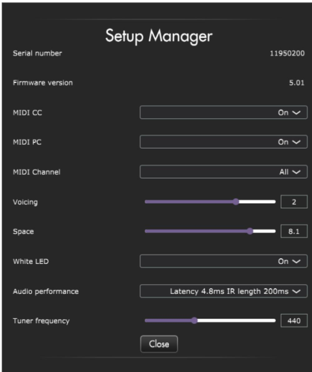
This section of Torpedo Remote sets the hardware parameters of the unit such as the audio latency, the MIDI mapping, the white LED, etc. You will also find the serial number of the unit, as well as the firmware version. You will also set the reference point for the tuner. By default, it is set at 440 hz.
