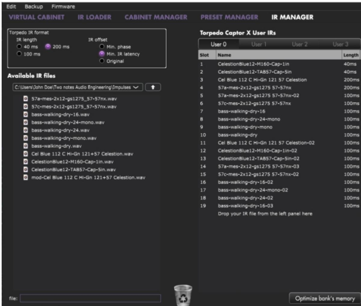
The left panel is the files on your computer. You can browse the folders where you have stored your IRs. The right side represents the IR files that are loaded in the Torpedo Captor X. You can drag and drop the IRs from the computer (left) to the Torpedo (right). If you wish to free memory slots in the pedal, you can drag and drop the IRs to the bin at the bottom. (this does not delete the IR from your collection, only from the Torpedo Captor X).
