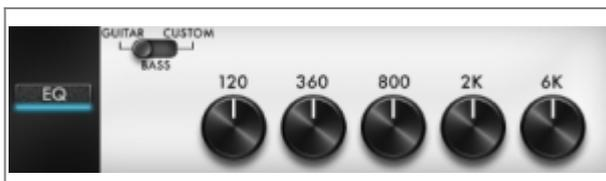
The EQ section has 3 modes of operations: guitar, bass and custom. Guitar and Bass are 5 band eqs, with a gain range of -20dB to +20dB. The Custom mode gives you access to a 5 band semi parametric eq and a high pass filter.
