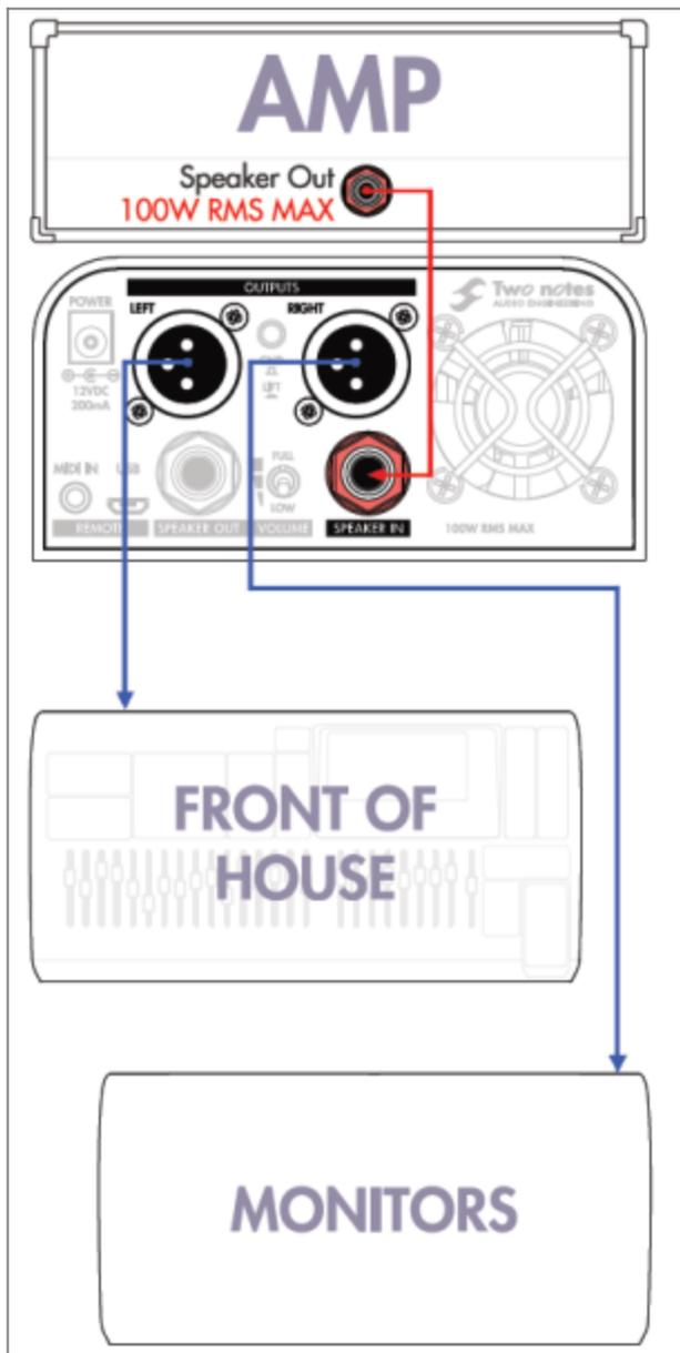
Connect your amp's output to the SPEAKER INPUT of the Captor X, indicated by a red bolt - ONLY use a speaker cable for this connection. In Torpedo Remote, select the DUAL/MONO routing to send 2 different signals from the Torpedo Captor X. Use microphone cables to connect to the Front Of House and the Monitors' mixing desk. You can connect your cabinet to the SPEAKER OUT if you wish to hear your dry amp sound on stage.
