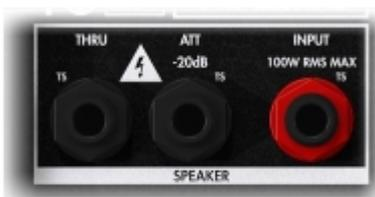
The speaker output of the amp connects to the SPEAKER INPUT of the Captor. You can't miss this input : it's the one with the red nut. Use a standard speaker cable for this connection (a pair of insulated conductors with no shielding).
