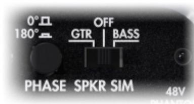
The speaker simulation embedded in the Captor is taken from our Le Preamp series. It's an analog simulation, featuring two models, Guitar and Bass, based on our Torpedo simulator. The Guitar model is based on our classic Brit VintC 4×12 picked up with a Dyn57. The Bass model is based on a mix of the vintage Fridge 8×10 and more modern Alu XL 4×10, picked up with a Cnd87.
