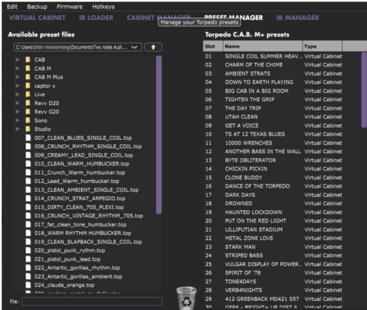
Move the presets up and down to change their order in Torpedo C.A.B. M+. The first 6 slots are accessible by the PRESET knob at the front of the unit. Remove presets by dragging and dropping them in the bin below. Drag and drop presets from the left panel (your computer) to the right panel (internal memory of the C.A.B. M+).
