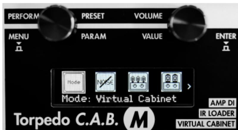
To enter any section and edit the related parameters, scroll to the relevant section by turning the PARAM encoder and press ENTER to enter. Some sections can be modified directly without entering it, by turning the VALUE encoder. For most of them, this means turning it ON or OFF (the image will then appear in negative mode).
