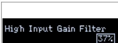
The Torpedo C.A.B. M+ firmware provides a clean foundation tone for your pedalboard. For optimal results, we advise setting the IN LEVEL switch at 0 dB. In the event you wish to use your guitar straight into the C.A.B. M (upgraded with the C.A.B M+ firmware) and boost the input with the +12dB, we provide a filter to keep your tone as pure as possible from any parasitic noise. This filter is set at 37% by default.
