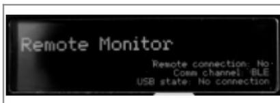
This menu indicates whether you are connected to the Remote or not and if you are connected to the Torpedo C.A.B. M+ by USB or by Bluetooth (BLE). This can be used to troubleshoot communication issues with the Remote and Wireless Remote software.
