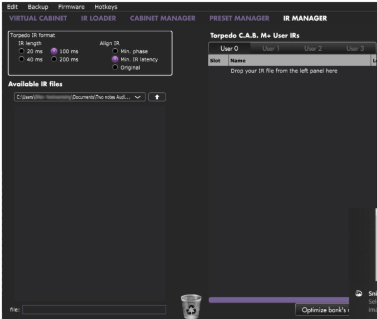
The left panel is the files on your computer. You can browse the folders where you have stored your IRs. The right side represents the IR files that are loaded in the Torpedo C.A.B. M+. You can drag and drop the IRs from the computer (left) to the Torpedo (right). If you wish to free memory slots in the pedal, you can drag and drop the IRs to the bin at the bottom.
