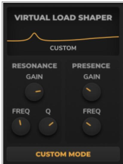
The **VIRTUAL LOAD SHAPER** is accessible from both the **VIRTUAL CABINET** and **IR LOADER** windows, and operates as a global parameter, with its settings applied across all presets on the Torpedo Captor X +.
