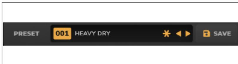
The Preset Rack, located at the top of the **VIRTUAL CABINET** and **IR LOADER** windows, allows you to save and load presets within the Torpedo Captor X +. The unit provides 128 memory slots for storing your custom presets.
