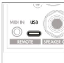
To connect the Torpedo Captor X + to your computer, use the supplied USB cable. Plug the USB-C end into the Captor X + and the other end into your computer's USB port.
