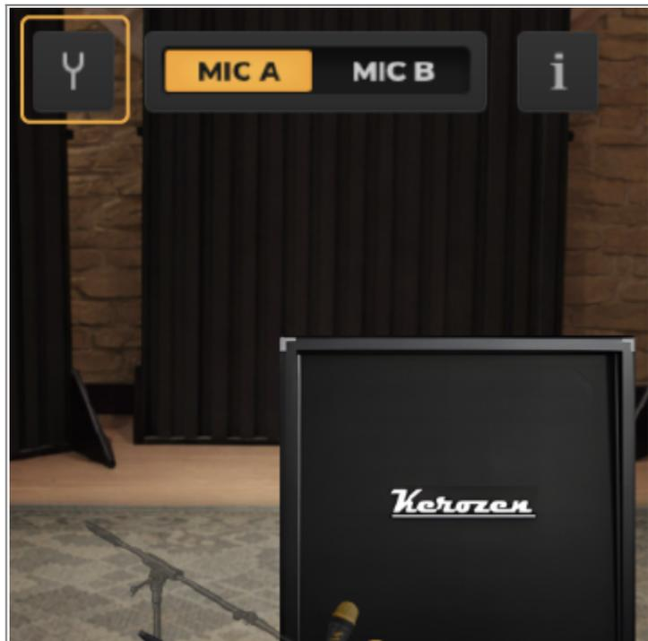
Access the **TUNER** by clicking the fork icon located next to the mic selection in the Room image. The tuner is fully chromatic, and its reference pitch can be adjusted in the [SETUP MANAGER](#) from 410 Hz to 490 Hz, with a default of 440 Hz.
