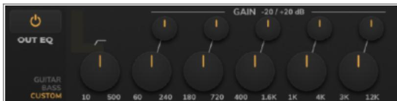
In the **DUAL/MONO** output routing mode, the Torpedo Captor X + provides a dedicated **OUTPUT EQ** for each XLR output.
