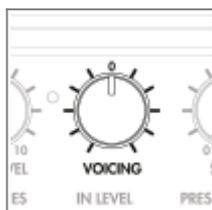
On the front panel of the Torpedo Captor X +, the **VOICING** control shapes the overall tonal balance of the signal routed to the XLR outputs. It operates as a single-band EQ centered at 900 Hz, offering a -12 dB to +12 dB adjustment range.
