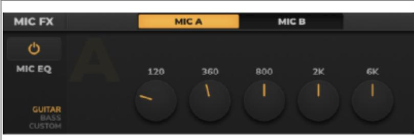
In the both the **VIRTUAL CABINET** and **IR LOADER** modes, the Torpedo Captor X + provides channel-specific **EQs** for each DynIR microphone (**VIRTUAL CABINET** Mode) or loaded Impulse Response (**IR LOADER** Mode), allowing precise tonal shaping of individual channels.
