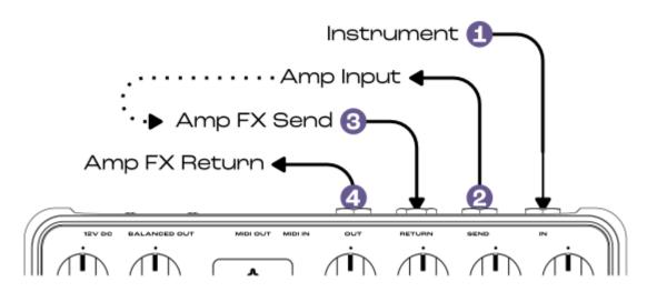
If your amp is equipped with an effects loop, add ReVolt's 3 channels to your amplifier's channel specification. Engage the 4-CABLE METHOD on ReVolt, and combine ReVolt's effects loop with the amp's using the following connectivity guidelines.
