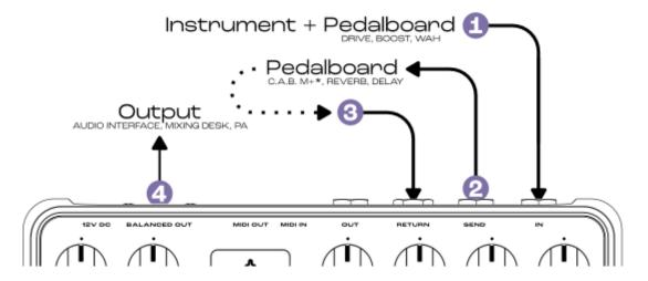
Use ReVolt to go-direct to mixing desks audio interfaces when on stage or recording respectively.
