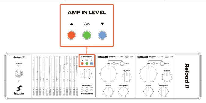
Located on the front-plate of Torpedo Reload II is the AMP IN LEVEL controls (Knob & LED Indicator). Correct configuration of this input-centric control is vital when priming any Amplifier to leverage all the might Reload II's dual 215W per-channel power amplifier delivers. When connecting an amplifier, first set the level using the AMP IN LEVEL knob, ensuring the source level falls within the "OK" range, highlighted via the related LED indicator.
