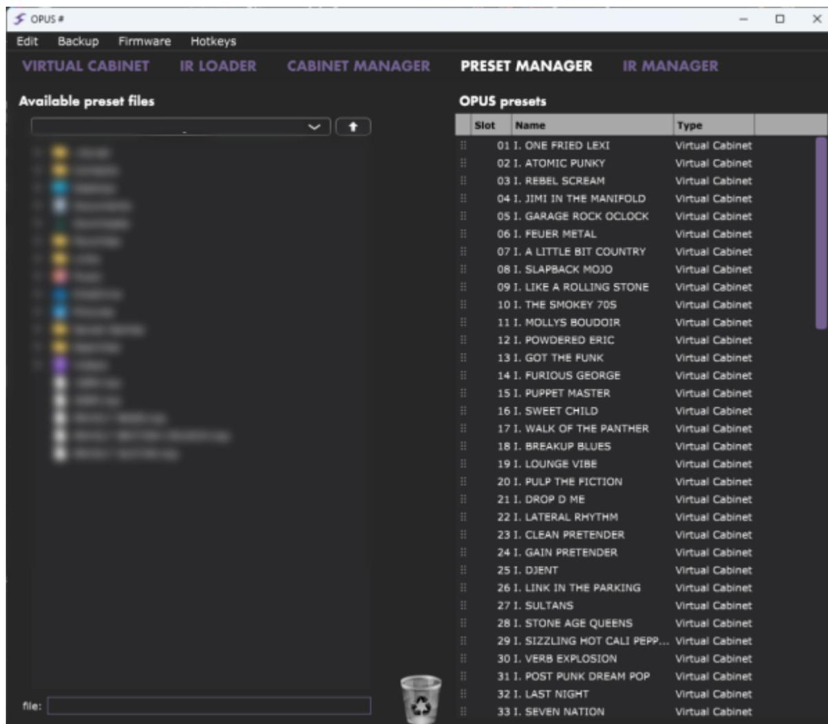
Move the presets up and down to change their order in OPUS. Remove presets by dragging and dropping them in the bin below. Drag and drop presets from the left panel (your computer) to the right panel (internal memory of the OPUS) to transfer presets from your computer to the OPUS hardware.
