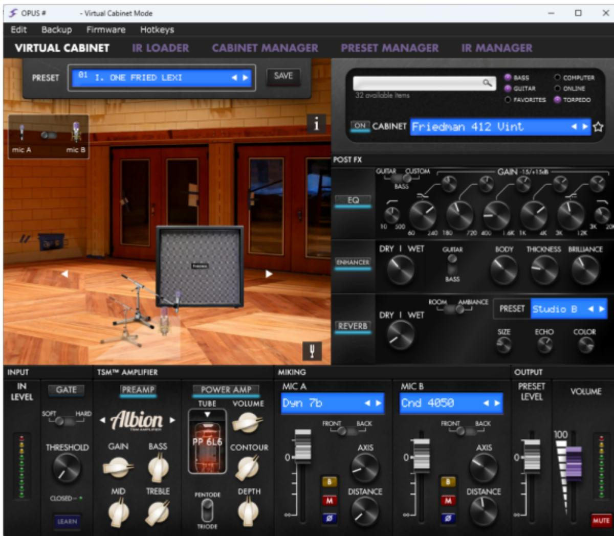
The main window of Torpedo Remote provides access to all of OPUS' tone shaping tools, as well as preamp, poweramp, cabinet and mic choice. This is also where you will manage the internal memory of the unit via the tabs located at the top of the window.
