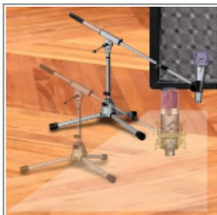
You can move the microphones anywhere in the trapezoid highlighted area as shown within the miking pane of the Torpedo Remote DynIR™ graphical user interface. Select MIC A or MIC B via the dedicated switch and move the microphone with your mouse (when using a computer) or your finger (when using a mobile device) by pressing on either the microphone image or the associated mic stand.
