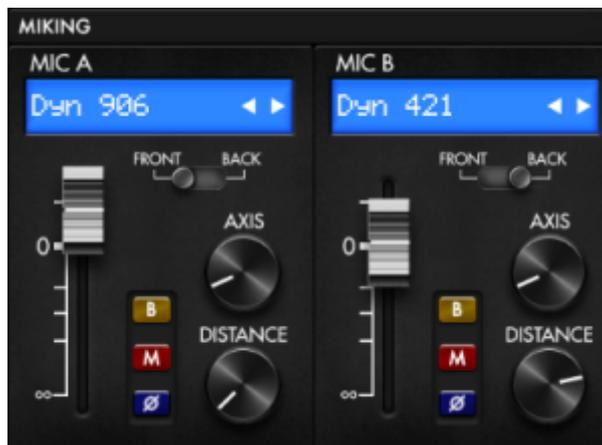
All Two notes Virtual Cabinets come with an individual collection of 8 microphones specifically matched to the cabinet. You access the list of microphones by clicking the blue window above the mic channel fader. For easy identification, microphones are described by their underlying technology: **DYN** is a dynamic microphone, **CND** is a condenser microphone and **RBN** is a ribbon mic.
