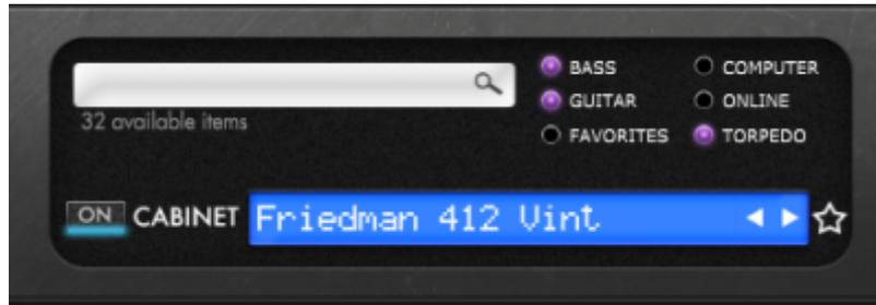
To create a foundation tone for your preset, first select a preamp, a poweramp and a cabinet. OPUS comes with a collection of 32 DynIR™ Virtual Cabinets preloaded into the internal memory. OPUS has a total of 64 slots in its internal memory for DynIR cabinets. Click on the blue screen or the drop-down arrow to access the list of cabinets preloaded within OPUS. Using Torpedo remote's filtering options, you can:
