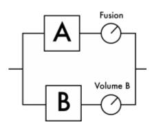
The Cold Fusion puts the Channels A and B in parallel. In other words, you will be able to adjust the level of Channel A that will be added to the output of Channel B. This technique consisting in adding a clean signal to a more distorted one is widely used in the studio to regain dynamics and articulation when the dirty sounds can be too compressed for example. The Fusion knob must be carefully adjusted and we recommend starting very low on this value and increasing gradually.
